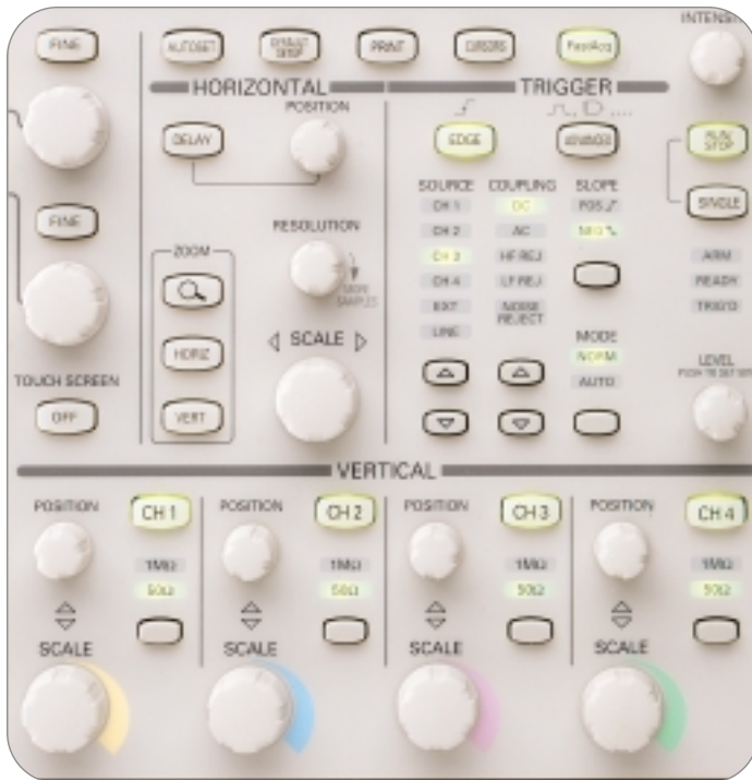
► Figure 22. Front-panel control section of an oscilloscope.
